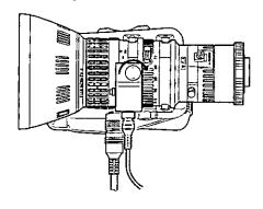
3 Install the zoom controller on the right tripod arm and the focus controller on the left tripod arm.
