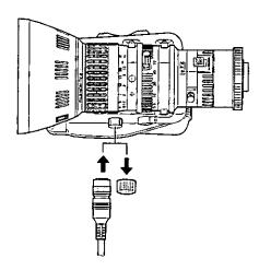
2 Install the gear box on the lens and connect the flexible cable to the gear box and the focus controller.
